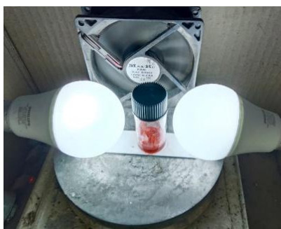
Figure S1. Photochemical reaction set-up
