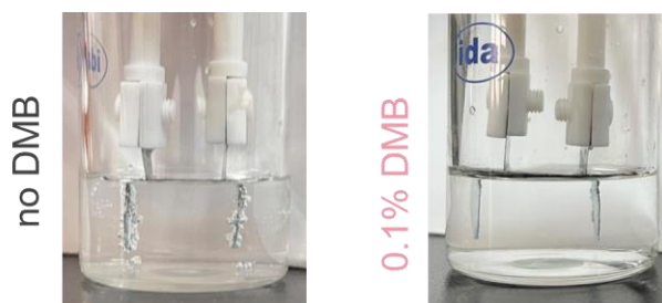
Fig. S6. Optical images of Zn plating/stripping in beaker cells at the 50th cycle in the \text{ZnSO}_4 electrolytes (a) without and (b) with the DMB additive.
