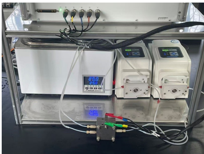
Fig. S17 The schematic diagram of the AEMWE system using Pt/C|| Ni 2 P/Fe 2 P-Ga 0.1 .
