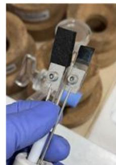
The starting material **1a** was fully decomposed, and no formation of the desired product **2a** was detected. A black passivation layer was formed on the Pt plate counter electrode.
