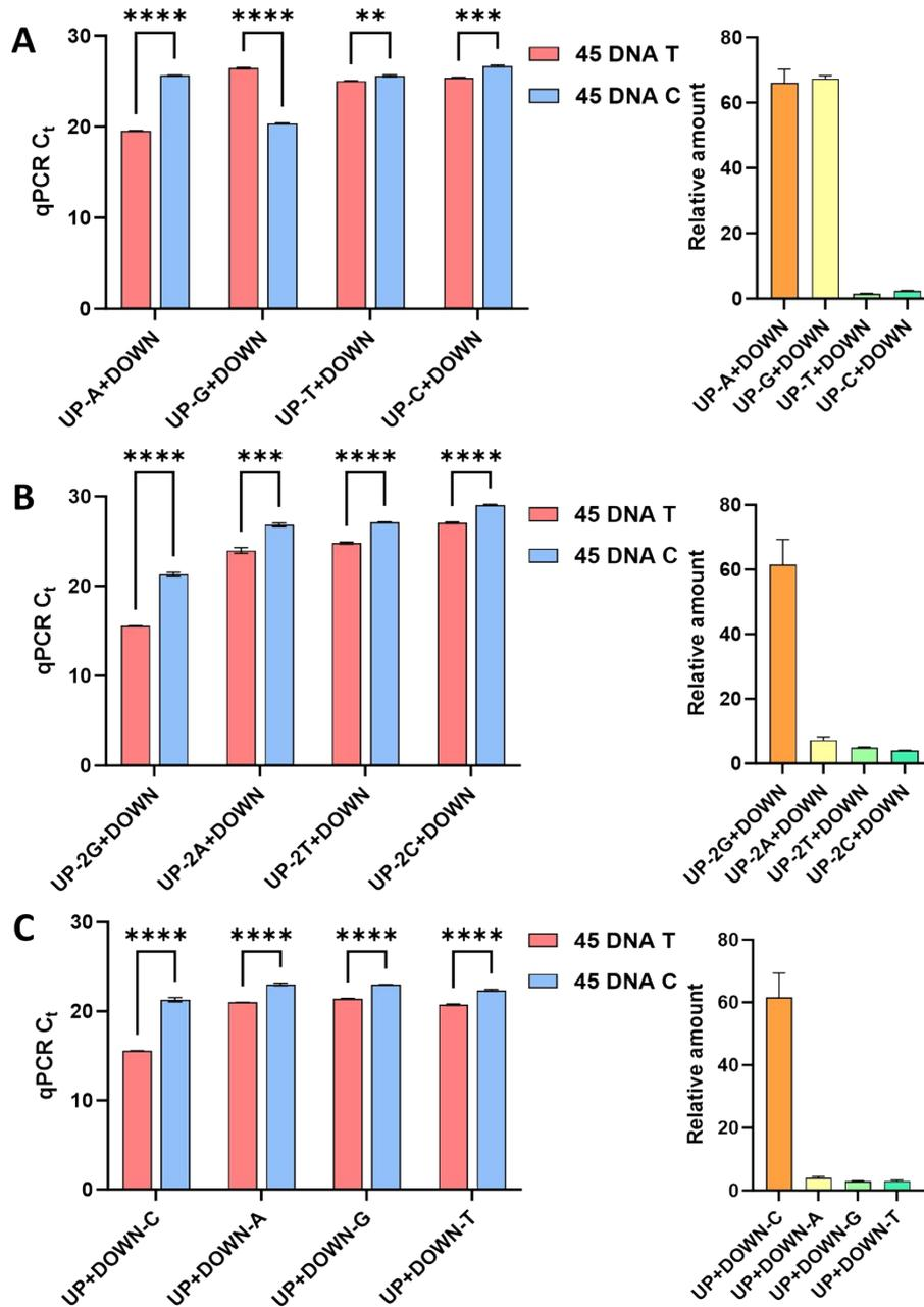
**Figure. S2** Impact of terminal base mismatches in UP and DOWN probes on the generation of ligation products. **(A)** Altering the terminal base of the UP probe. **(B)** Altering of the penultimate base in the UP probe. **(C)** Altering the terminal base of the DOWN probe. 10 ng DNA was carried out for analysis. Error bars indicate mean  $\pm$  s.d. for three technical replicates. \*P < 0.05; \*\*P < 0.01; \*\*\*P < 0.001; ns, non-significant by t-test (two-tailed).
