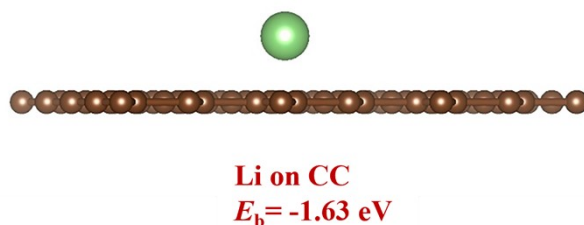
Fig. S9 Calculation of binding energy of Li with graphitic carbon.
