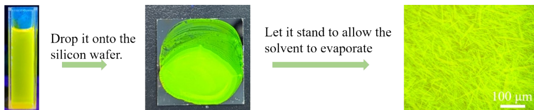
Figure S9: Photos of the assembly process. Place the silicon wafer on the desktop. Take 30 microliters of NPLs solution (20 mg/ml), drop it onto the silicon wafer, and keep it still until the solvent evaporates completely.
