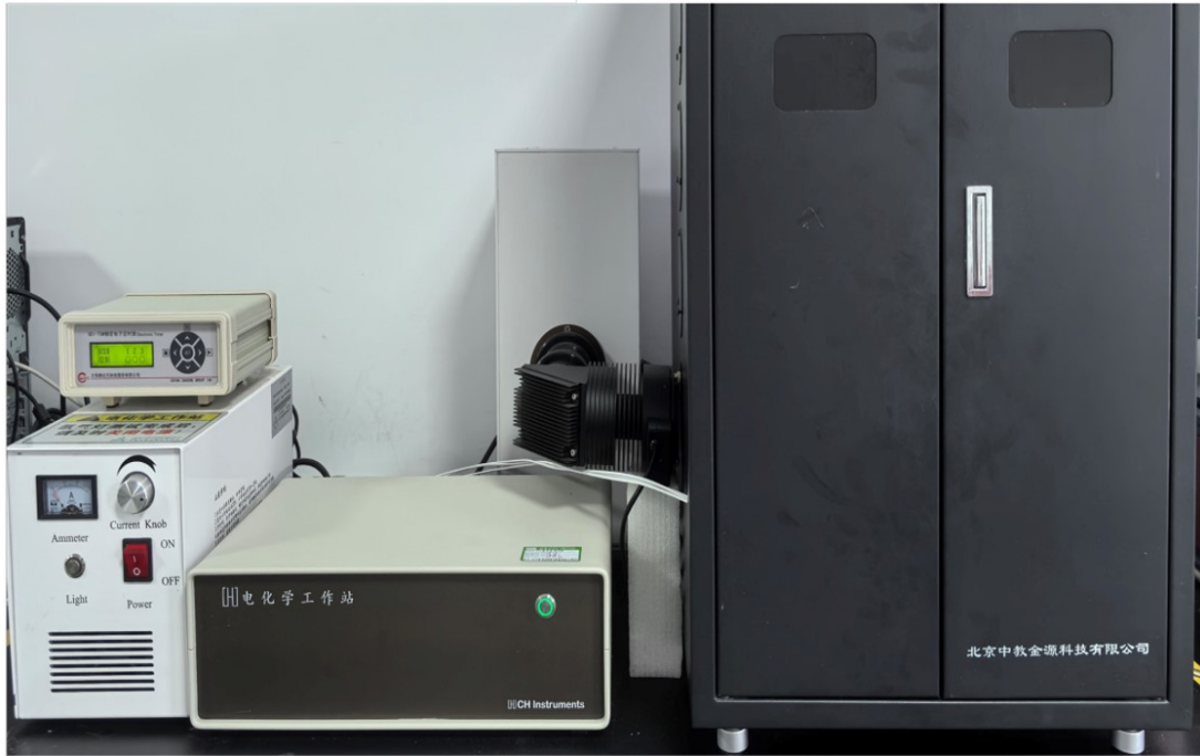
Fig. S2. Optical image of a three electrode photoelectrochemical measuring device
