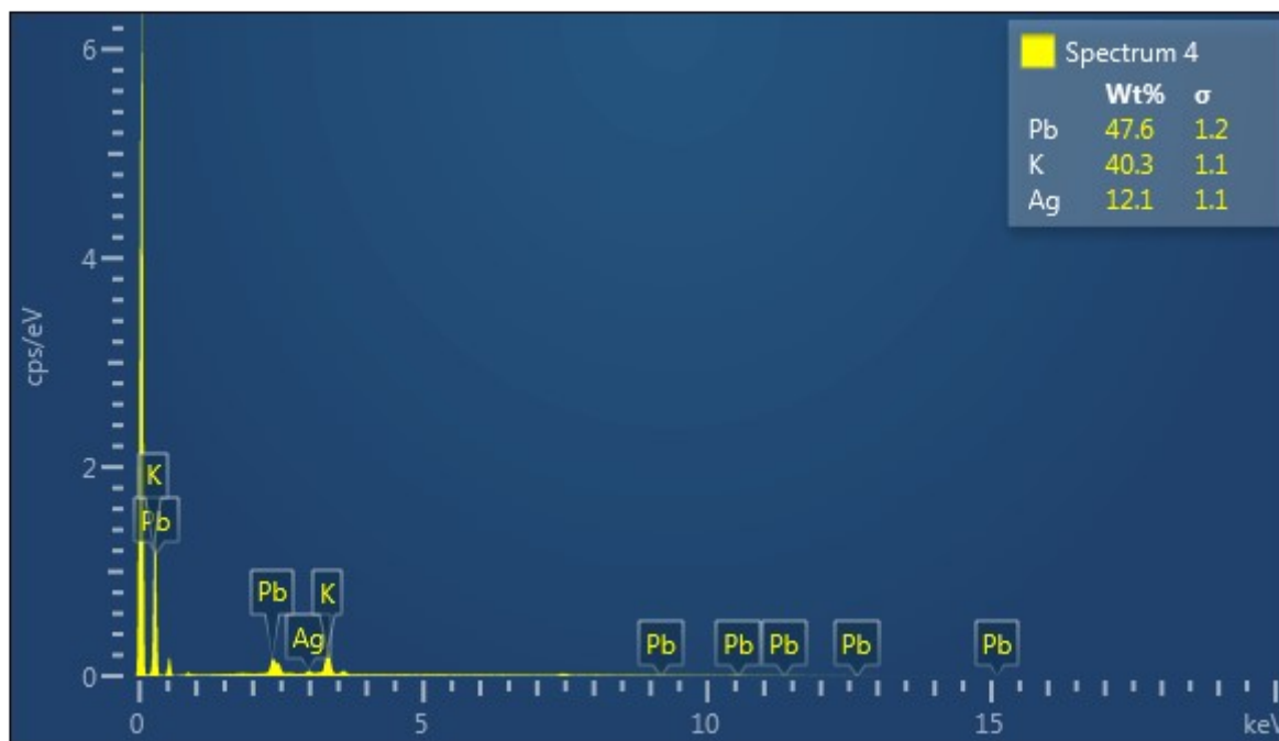
Figure S6. EDX analysis of complex \text{K}([\text{2.2.2}]\text{crypt})_3[\text{Ag}@\text{Pb}_{12}]\cdot\text{tol} ( 1 ).
