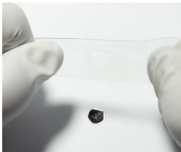
Figure S3. Delamination of the PVB reference membrane. Optical image showing the PVB membrane detaching from the TPU substrate during mechanical deformation, indicating poor interfacial adhesion and mechanical incompatibility with the stretchable substrate.
