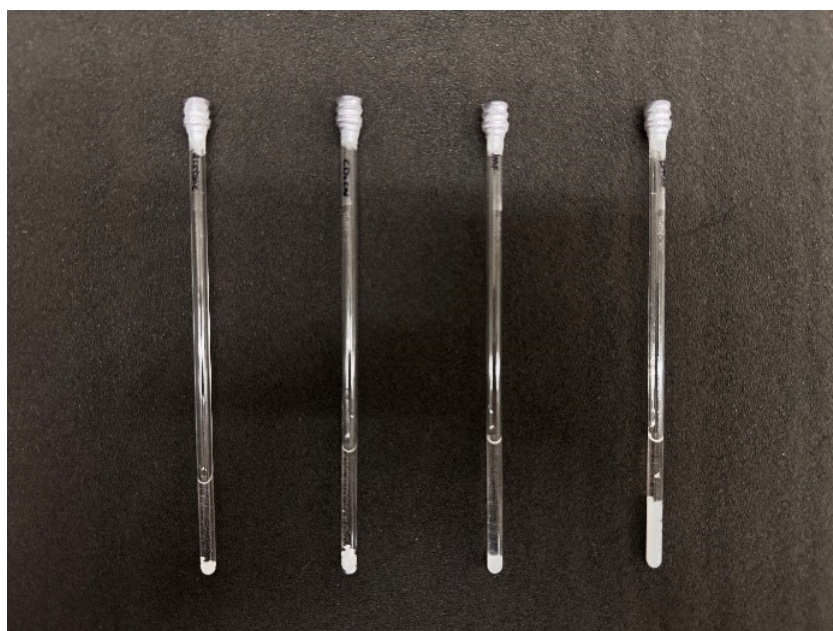
Figure S1. NMR samples containing deuterium solvents and PBLG after mixing, from left to right a) Acetone- d_6 with 0.6% (w/v) PBLG, b) \text{CD}_3\text{CN} with 1.3% (w/v) PBLG, c) DMSO- d_6 with 3.9% (w/v) PBLG, and d) DMF- d_7 with 4.0% (w/v) PBLG.
