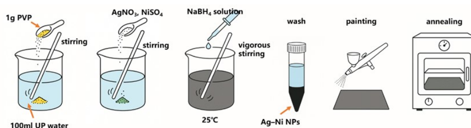
Fig. S1 Synthesis of catalyst and preparation working electrode.
