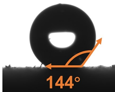
Fig. S14 Water contact angle image of PCNF-plasma (144°).
