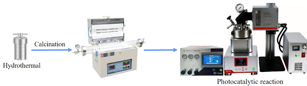
Scheme S1. Preparation process of S-TiO 2 and schematic diagram of the reaction setup.
