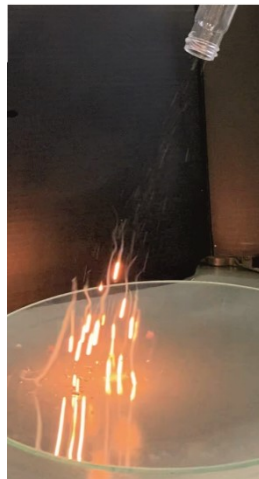
Figure S4. Photo illustrating the reactivity of Na(0) nanoparticles (10 mg) when in contact to air.
