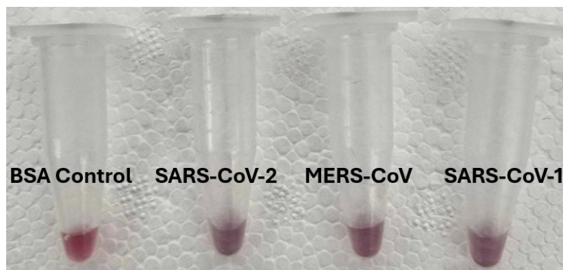
Figure S1. Specificity test for the S2A2C1 aptamer using an AuNPs-based colorimetric assay.
