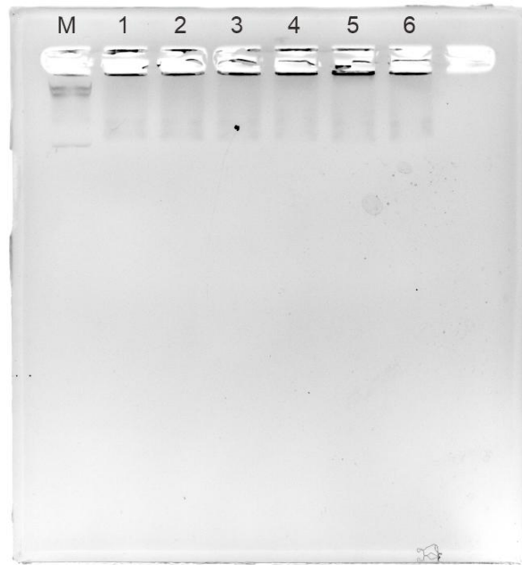
Supplementary Fig. 24. 1% Agarose gel electrophoresis analysis of ring-shaped DNA origami (RDO). Representative agarose gel electrophoresis of purified ring-shaped DNA origami after silicification at different silicification reaction temperatures. Lanes from left to right correspond to 1kb DNA ladder, pristine ring-shaped DNA origami (10 nM) and ring-shaped DNA origami (10 nM) silicification at 4, 15, 25, 37, and 45 °C, respectively.
