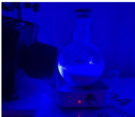
Figure S2. Photoreaction set-up for scale-up reaction.
