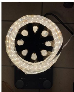
(i) Designed vial stand inside the photoreactor for multiple reactions
