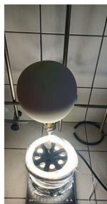
(f) Reaction vial under irradiation (front view & top view)
