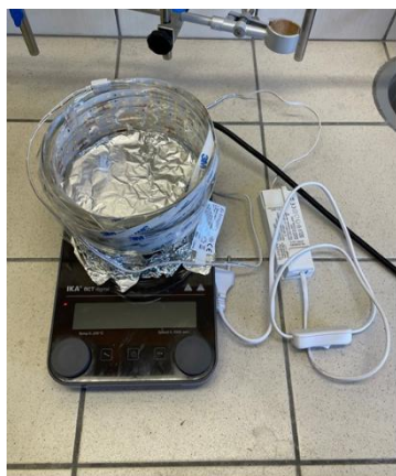
(a) Designed photochemical reactor with LED stripes
