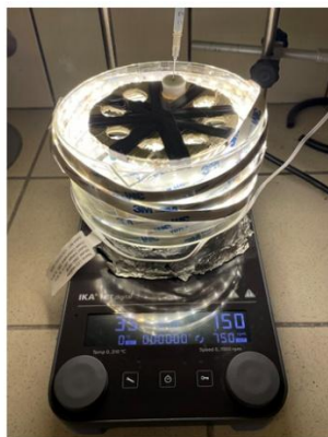
(f) Reaction vial under irradiation (front view & top view)
