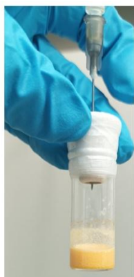
(e) Reaction vial charged with reagents & degassed by sparging with argon
