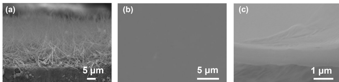
Fig. S1. The SEM images of (a) the cross-section of MIL-110 skeletons, (b) the surface and (c) the cross-section of the SPEEK membrane.
