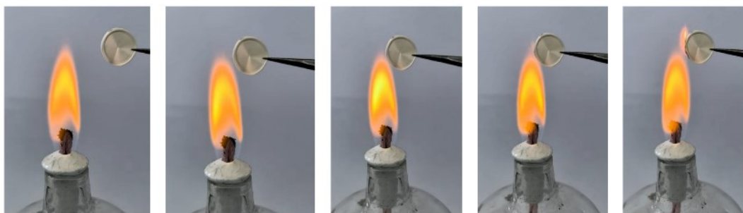
Figure S6 Flame test of the Si-HOF-based SSEs.
