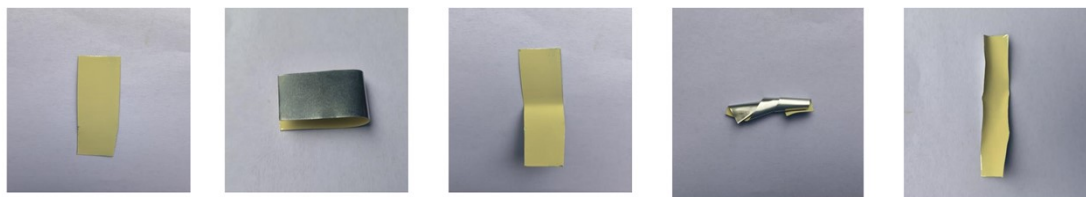
Fig. S5 Photographs of Cu@g-C 3 N 4 @Zn under bending and twisting tests, demonstrating the mechanical flexibility and interfacial adhesion of the coating.
