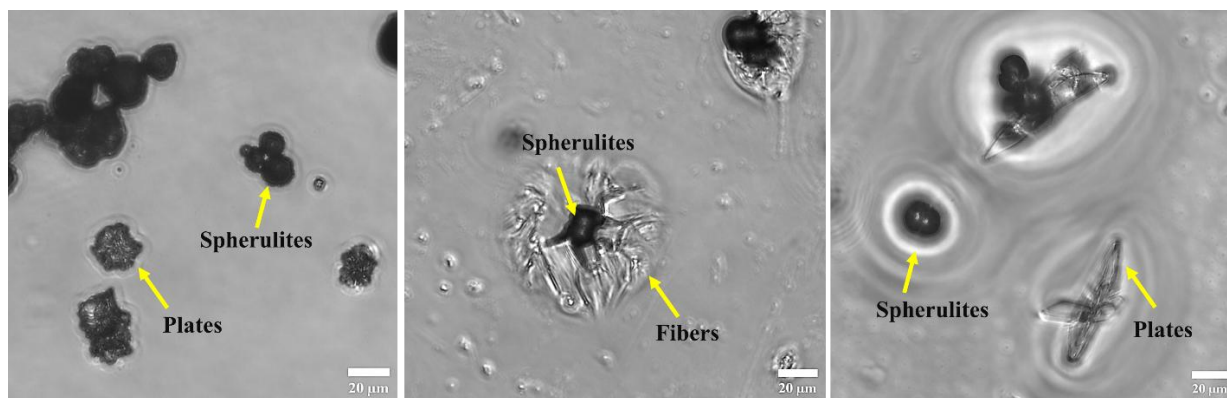
Figure S15. Optical micrographs showing formation of spherulites in all three basic medium along with other morphologies such as radially arranged plates in LiOH, fibres in NaOH and plates in KOH
