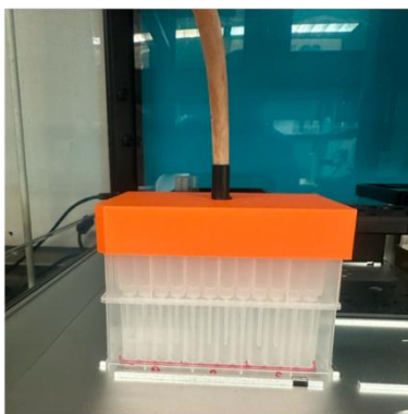
Figure S5: filtration set-up showing filter, receiver and our customized manifold for delivering overhead pressure to the filter apparatus
