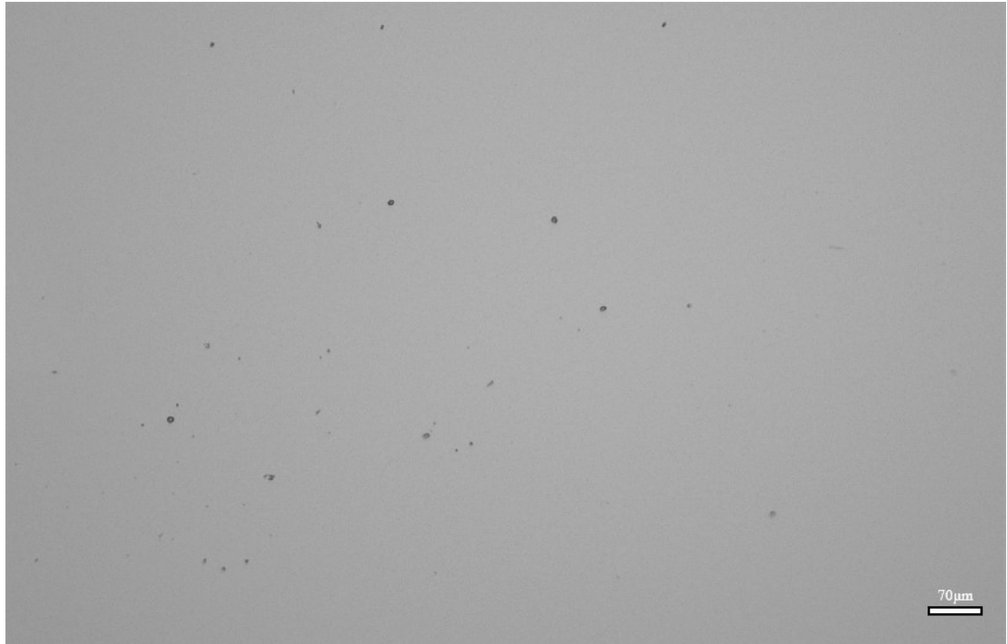
Fig. S3 Optical microscope image of the (010)-oriented surface etched in mixed solution of HF and HNO 3 at 60 °C for 4h
