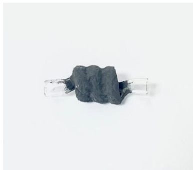
Fig. S11 (a) Carbon black powder coating disc device, (b) Carbon black powder coated conical component device, (c) Carbon black powder coated spiral component device.
