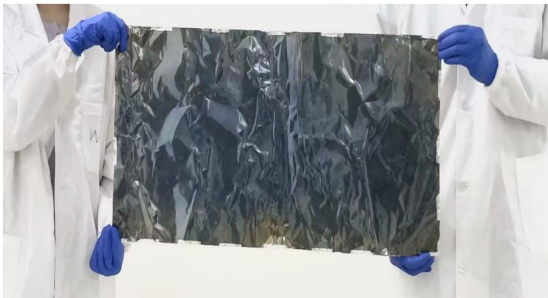
Fig. S10 The photograph of 150 nm MXene/Al film with large scale.
