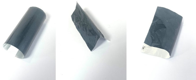
Fig. S9 The photographs of 150 nm MXene/Al film with various nest fold shapes.
