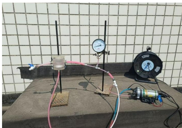
Fig. S1. Water treatment performance of the FeOOH/g-C 3 N 4 /CA catalytic membrane system under sunlight.
