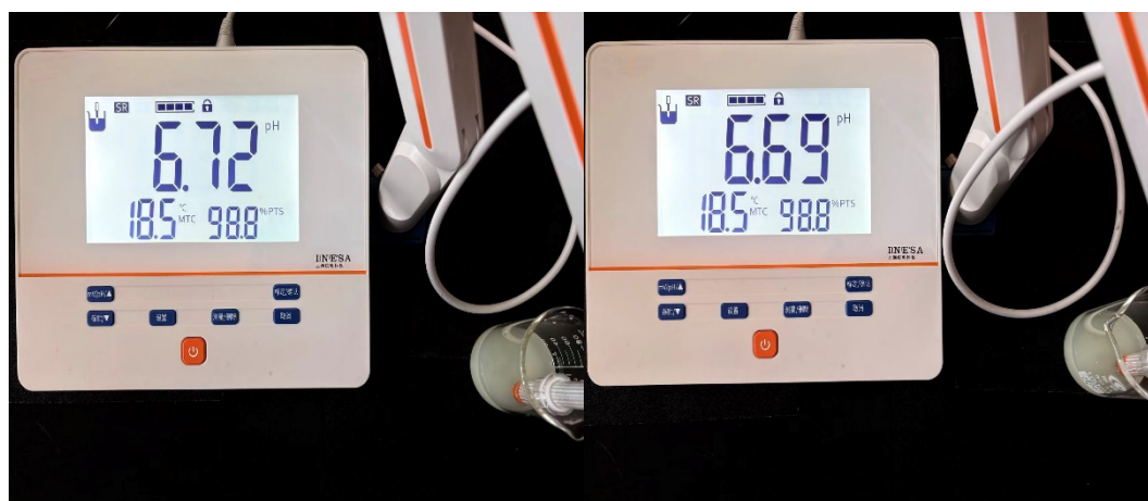
Figure S8. The pH value of solvent before and after H 2 O 2 photosynthesis.
