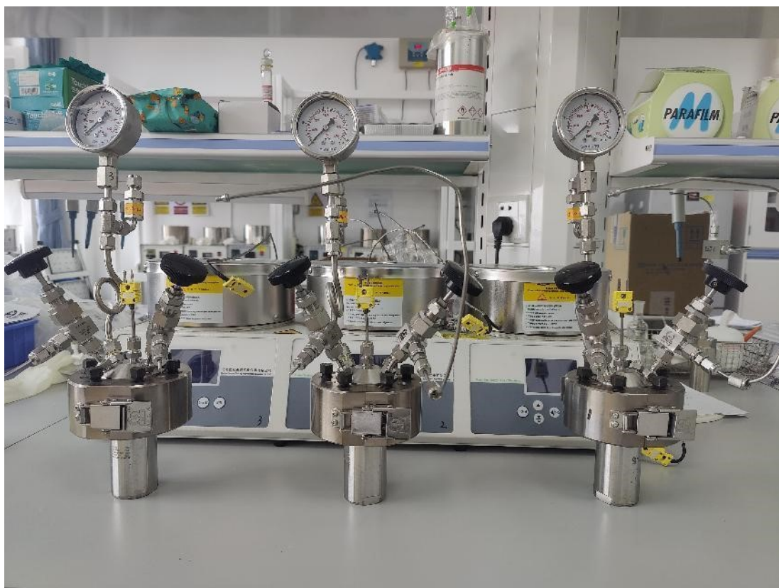
Fig. S9 The batch reactors with a capacity of 25 mL.
