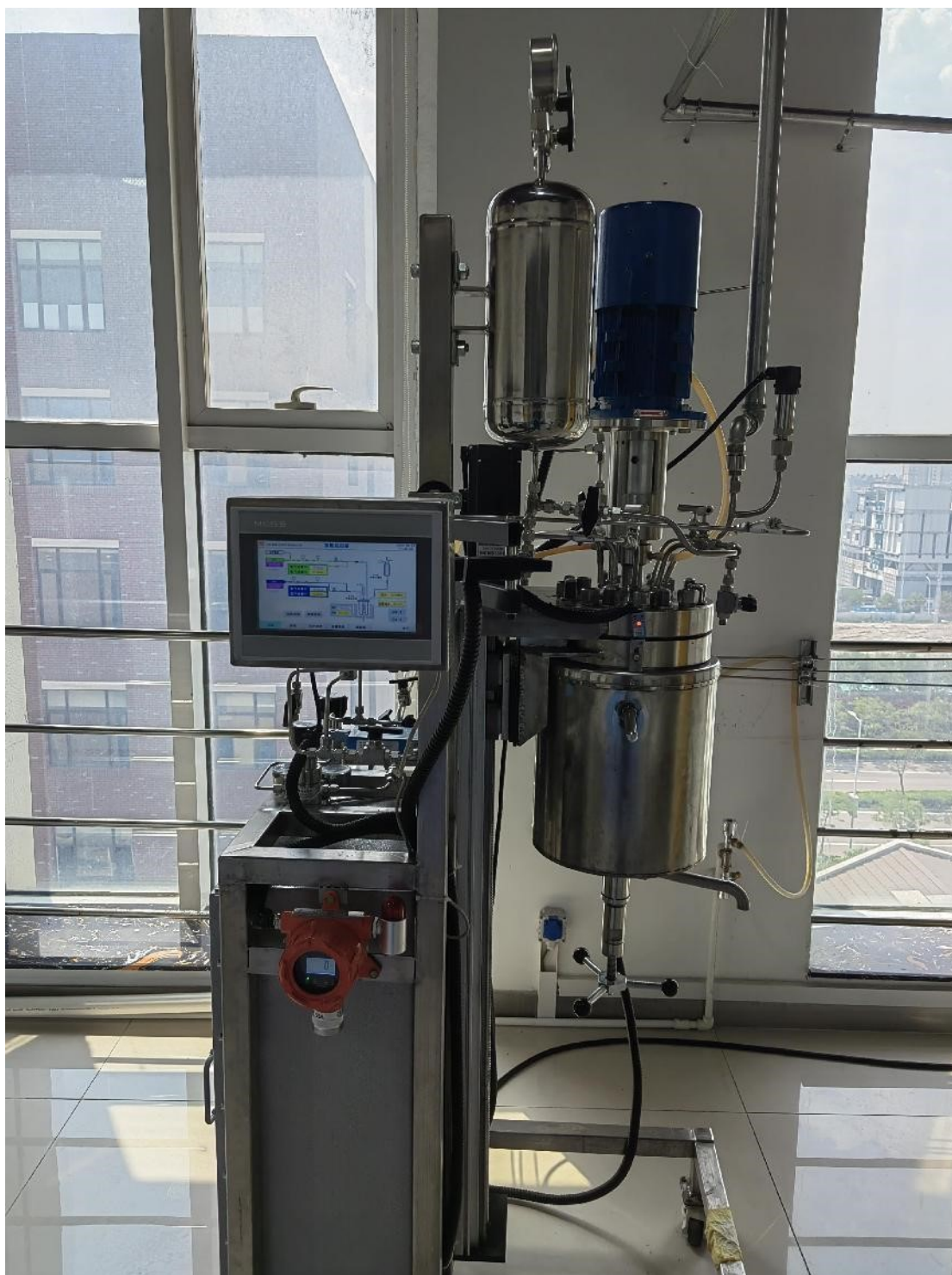
Fig. S10 The batch reactor with a capacity of 3 L.
