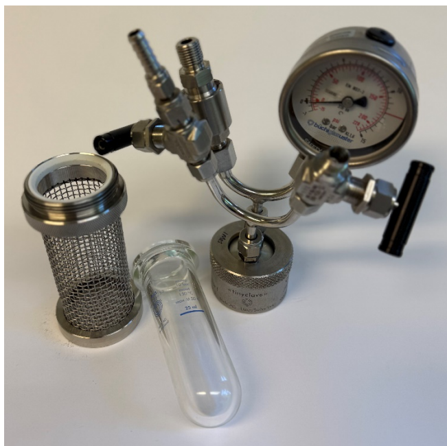
Figure S160. Büchiglass tinyclave glass pressure reactor.
