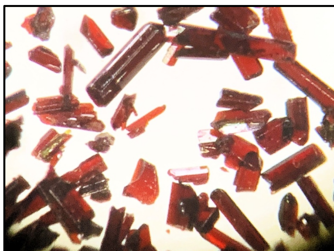
Figure S1: Picture of the as-synthesized reddish-brown rod-shaped crystals (under microscope) of [\text{Fe}(3\text{-bpp})_2][\text{Cr}(\text{ox})_3](\text{ClO}_4) \cdot 5\text{H}_2\text{O} (Compound 1) grown via liquid-to-liquid diffusion.
