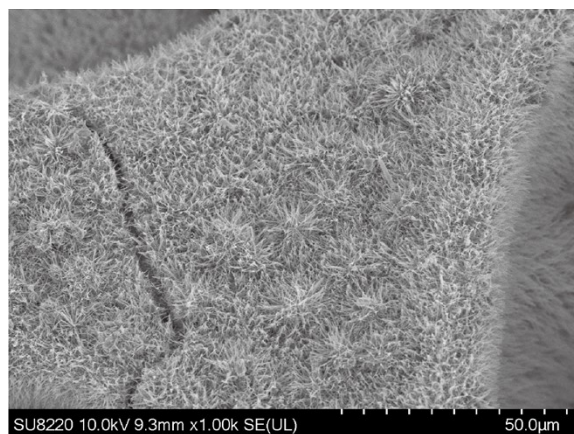
Fig. S3. The morphology of CuO/CF nanowires arrays grown on the copper foam at different magnification.
