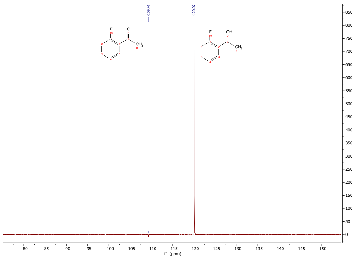
Figure S54 ^{19}\text{F}\{^1\text{H}\} NMR spectrum of reaction mixture following the TH conversion of 2-fluoro-acetophenone ( 1e ) to 2-fluoro-phenyl-ethan-(2)-ol ( 2e ) using Mn1d as (pre)catalyst
