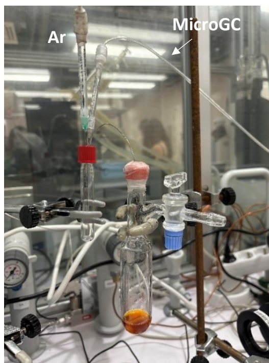
Figure S45 Experimental set-up used to detect hydrogen by GC-TCD.
