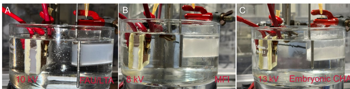
Figure S24. Photos of cuvette reactors during crystallization for different systems: A) FAU/LTA, B) MFI and C) Embryonic CHA.
