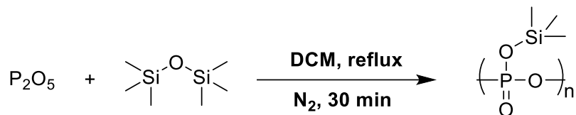
Fig. S3. Synthesis of the polymer PPSE
