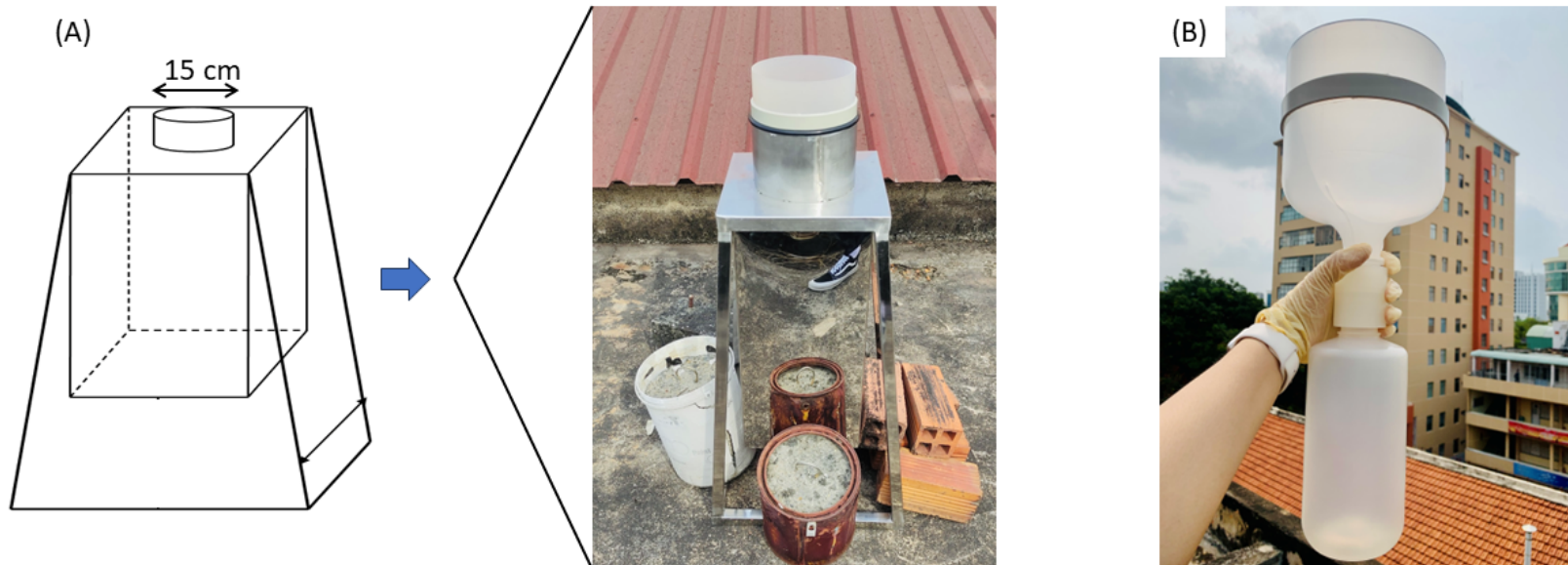
Fig. S2. Bulk deposition samplers used for rainwater collection in Ho Chi Minh City (A) Schematic diagram and actual device; (B) The HDPE sampler.
