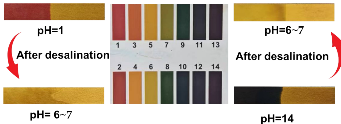
Fig. S55. pH values of acidic and alkaline solutions before and after purification.
