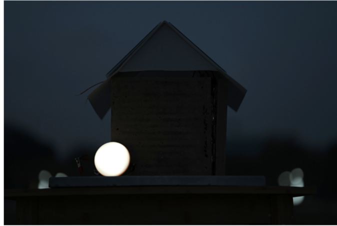
Fig. S28 The self-powered building demonstrator supplies electrical power to a light bulb during nighttime operation.
