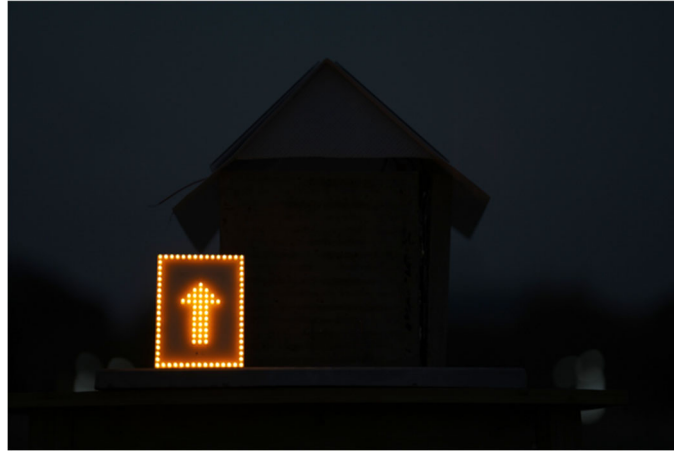
Fig. S29 The self-powered building model powers an illuminated 15 cm × 10 cm traffic sign during nighttime operation.
