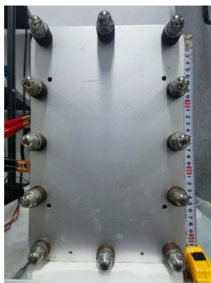
Figure S35. Large-sized battery with 1Mn+1Ti+3H electrolyte and N212 separator, showing its cycling performance and photos of the battery.
