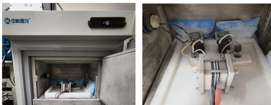
Figure S38. Schematic diagram and real-scene photos of the low-temperature testing device. (During the low-temperature battery test experiment, the peristaltic motor, the battery, and the electrolyte solution were all placed in the low-temperature box.)
