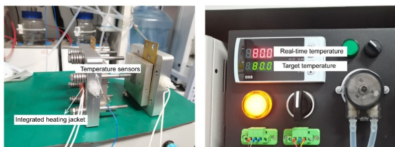
Figure S35. Temperature monitoring and real-time control system.
