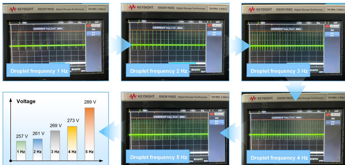
Fig. S28. Voltage curves recorded by an oscilloscope at different droplet frequencies.
