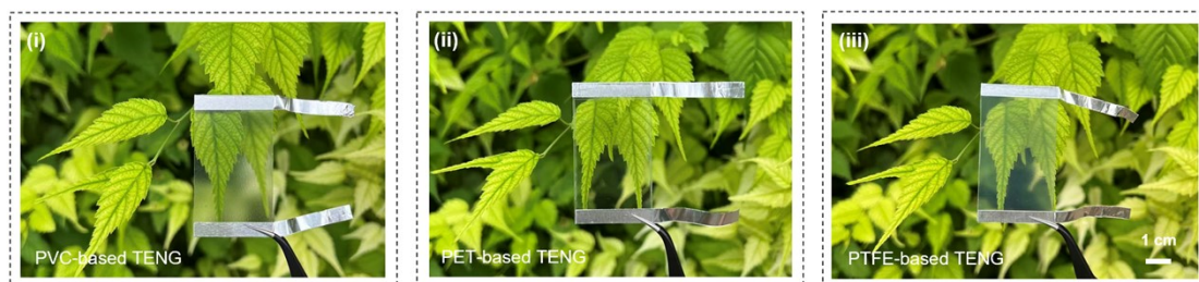
Fig. S25. Photographs of PVC-based TENG, PET-based TENG, and PTFE-based TENG under natural light.
