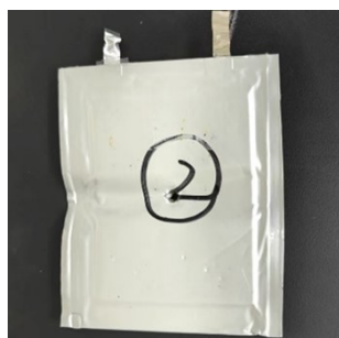
Figure S46. Optical photo of LFP||Li pouch cell after nail penetration.
