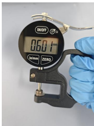
Figure S12. Digital-micrometer measurement of the HD-DESSs gel electrolyte thickness after absorption of the \text{Zn}(\text{OTf})_2 electrolyte solution. The final electrolyte thickness used for cell assembly was approximately 0.6 mm.
