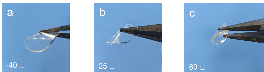
Figure S3. Optical images of gel electrolyte under a) -40\text{ }^{\circ}\text{C} , b) 25\text{ }^{\circ}\text{C} and c) 60\text{ }^{\circ}\text{C} .
