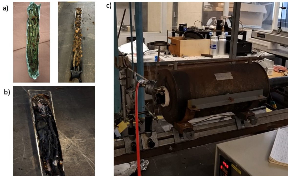
Figure 1SI: High-temperature combustion facility and post-combustion residues a) Samples in the sample holder before combustion, on the left for combustions up to 550°C, on the right for combustions at 800°C; b) Sample after combustion; c) Horizontal furnace used for controlled soil heating.
