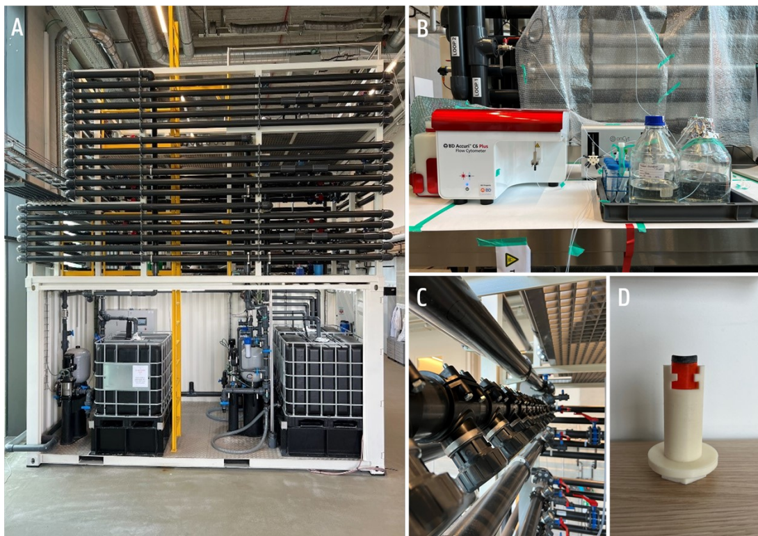
Figure S1: (A) The drinking water distribution pilot comprises three identical loops of 100 m each, connected to a non-translucent IBC. The structure measures 5.2 m × 2.6 m. (B) Implementation of online microbial monitoring: An Accuri™ C6 Plus flow cytometer (left) is coupled with an onCyt© autosampler, facilitating automated sampling from the pilot and cleaning solutions (right). (C) Biofilm sampling involves the use of coupons for undistruptive examination. These coupons are installed on a pipe using a system designed to resist pressure. (D) The coupon when removed from the pipe. It consists of a white holder (3.4 cm of diameter, 9.5 cm long), with a small insert (2.2 cm of diameter, 2.5 cm long) that can be placed within it. The top of this insert, which comes into contact with the water, is made of PCV-U, the same material as the pipes.
