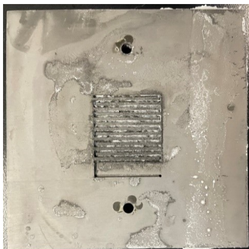
Figure S1. Postmortem of cathode flow fields after CO 2 RR test showing extensive precipitation after continuous operation at 200mA/cm 2 .
