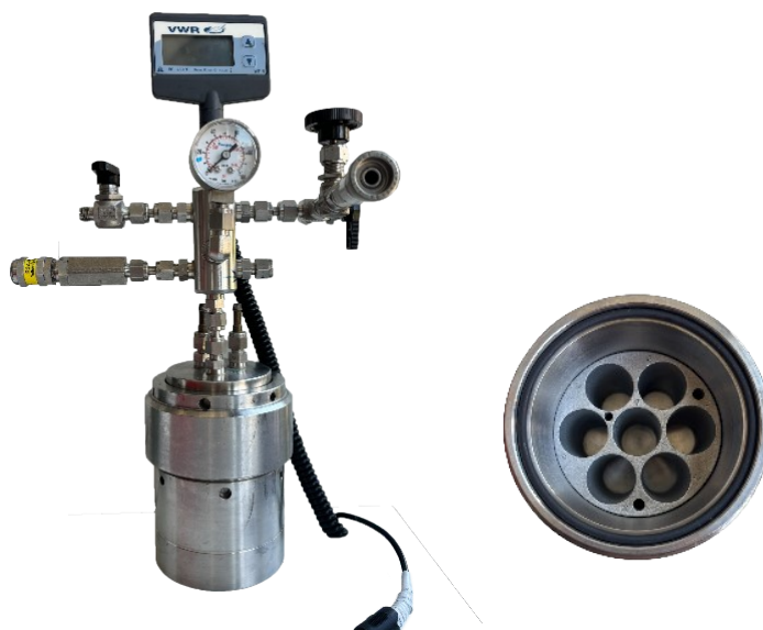
Figure S1. Custom high-pressure reactor used in this study. 7-well reactor (Alloy 600, reactor capacity: 483 mL). The pressure gauge is non-electronic and subject to error.
