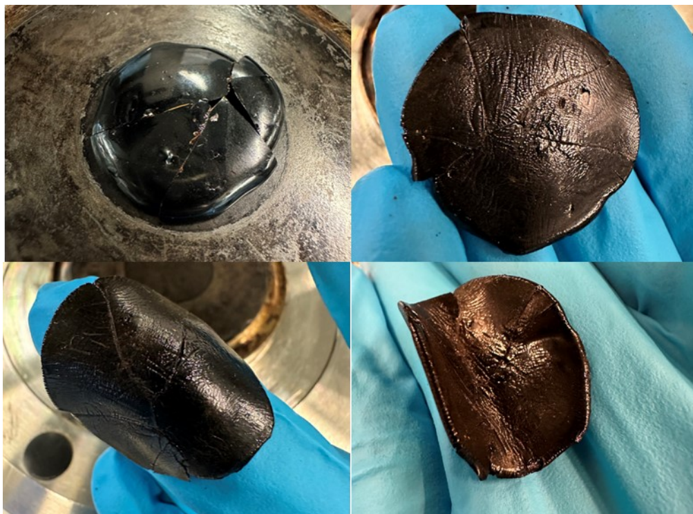
Figure S45. Self-healing behaviour of DDA4 solid on the rheometer plate at 60 °C for 10 minutes.
