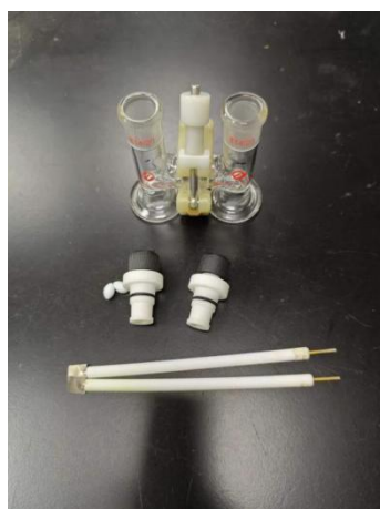
Figure S2. Electrochemical setup used for divided cell experiments.
